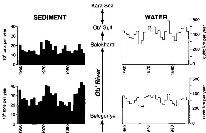
**Figure 5.** Annual water and sediment discharge in Ob' River, measured at Belogor'ye (upstream) and Salekhard (downstream). Our study area is situated between these two stations. Water discharge increases while sediment discharge decreases through reach. Figure was prepared by R. H. Meade, using data published by Bobrovitskaya et al. (1997).
