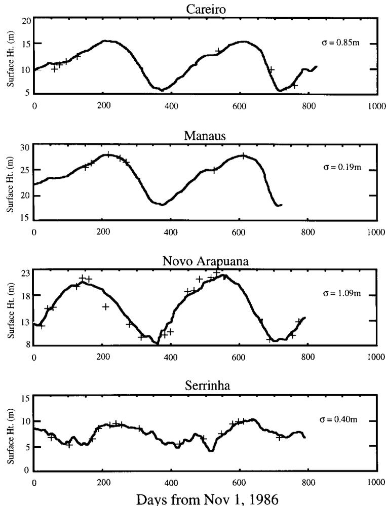
Figure 2. Comparisons in river stage at four sites in the Amazon basin, as estimated from river gauges (solid line) and Geosat altimeter waveforms (pluses). Standard deviations of the differences between the altimeter and river stage data are also shown. Period of observation is from November 1986 to November 1988. (Adapted from Koblinsky *et al.*, 1993)
