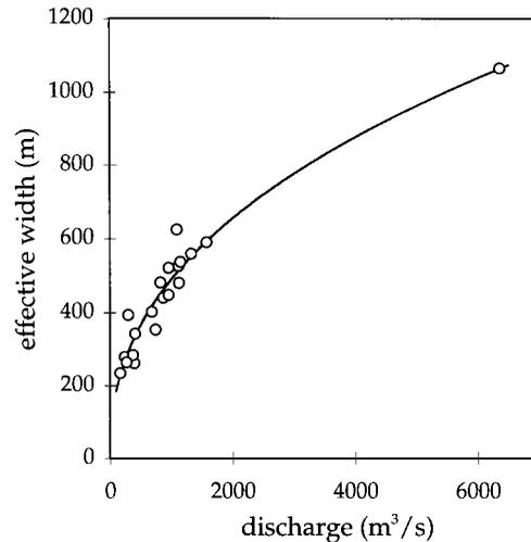
Figure 3. Relationship between satellite-derived effective width and river discharge for a large braided river in Canada. Effective width is the total water surface area contained within a 10 km  $\times$  3 km river reach, divided by the reach length. Each point is determined from a single ERS-1 SAR image and a ground measurement of discharge. The outlier is an extreme flood event; maximum annual flows do not normally exceed 2000 m<sup>3</sup>/s. (From Smith *et al.*, 1995)
